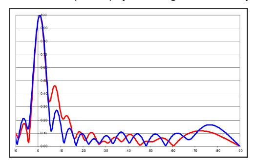
The plot above is a 16 element Vari-Phase antenna (RED plot) versus an 11 bay standard antenna (BLUE plot). The elevation gain of the Vari-Phase antenna above is 11.44 (10.58 dB) and has a 34% first null fill, plus the physical length of a 12 bay antenna.
