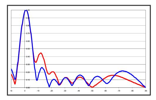
The plot above shows a elevation plot of a 10 element Vari-Phase antenna (RED plot) versus a 7 bay standard slot antenna (BLUE plot). Both have a beam tilt of 1.0 degree. The elevation gain of the Vari-Phase is 7.08 (8.50 dB), and has a 32.4% first null fill, plus a physical length of a 7.5 bay antenna.
